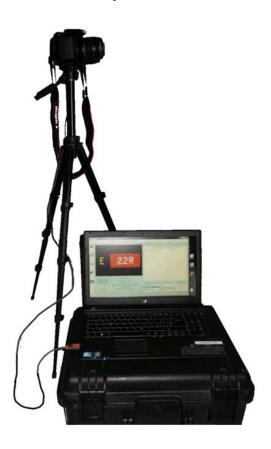
SMF/SIGN system is the fastest instrument for the in-field real-time assessment of Vertical Guidance Signs able to perform Luminance and Chromatic measurements with just a single camera shot.
